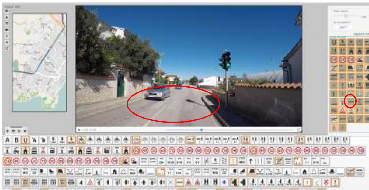
Video frame number 245777 at ŽC6086 (id 236): Recorded Pedestrian crossing - inspected road "signalized without a refuge" as "no facility"
